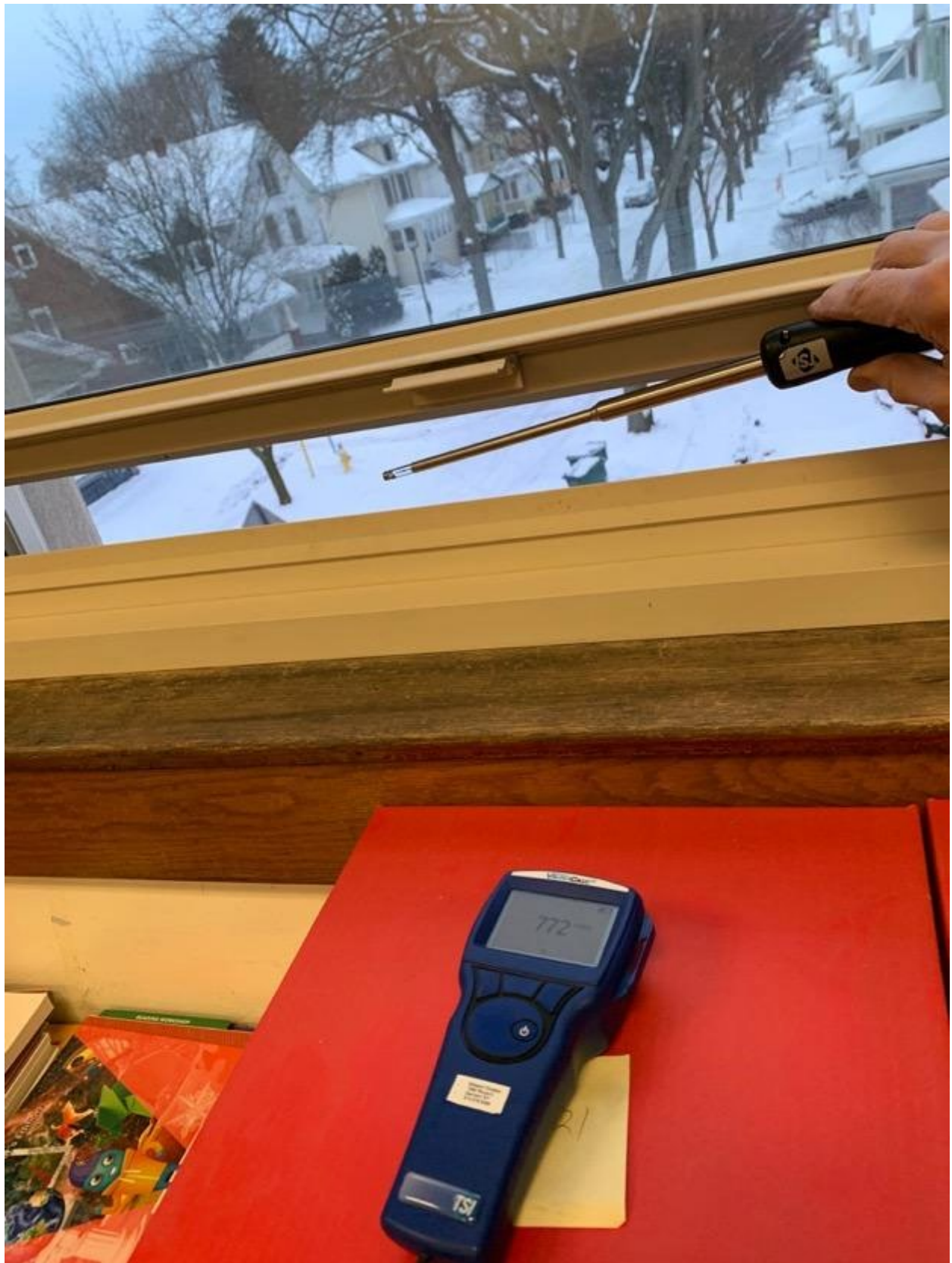
Testing of airflow through the open window provides 772 feet per minute
