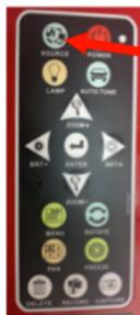
To switch between the Document camera and computer, press source
